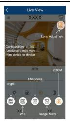
🕸: Zoom adjustment (this function is only available for cameras with motorized lens).
